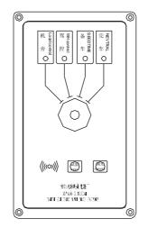
The content contacted via ATE is: transform for control position between wheelhouse control and local control, request and answer for SBE and FWE.
